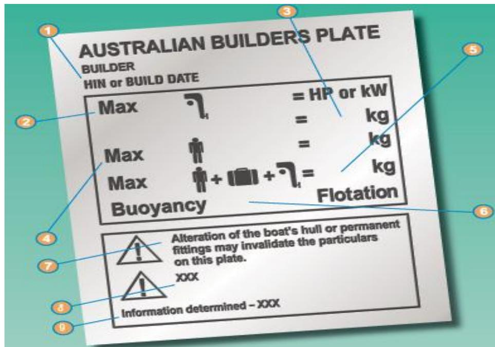
This is a sample of an ABP for a boat less than 6 meters with an outboard motor, as of 5 September 2005. For further details, please refer to the National Standard for Australian Builders Plate for Recreational boats
